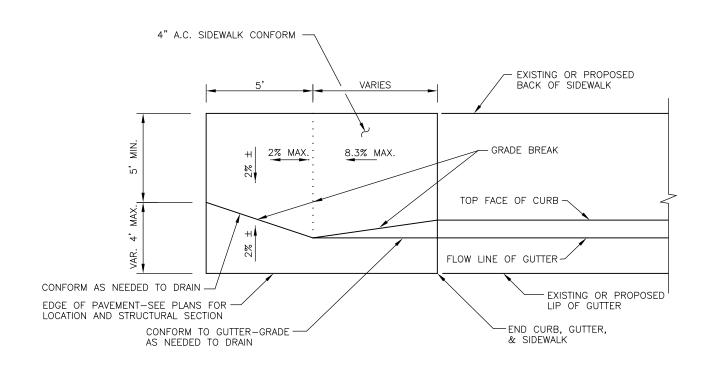
NOTE: A SIDEWALK BARRICADE SHALL BE REQUIRED IF THE END OF THE A.C. SIDEWALK CONFORM ABUTS A DRAINAGE DITCH OR ANY OTHER SURFACE THAT WOULD POSE A HAZARD TO PEDESTRIANS.
